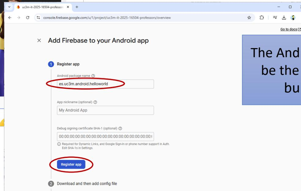
The Android package name must be the id defined in our app's build.gradle.kts
