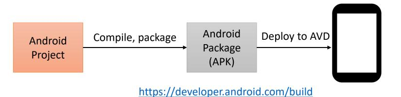
An APK is an archive file (.apk suffix) which contains the contents of an Android app that are required at runtime
